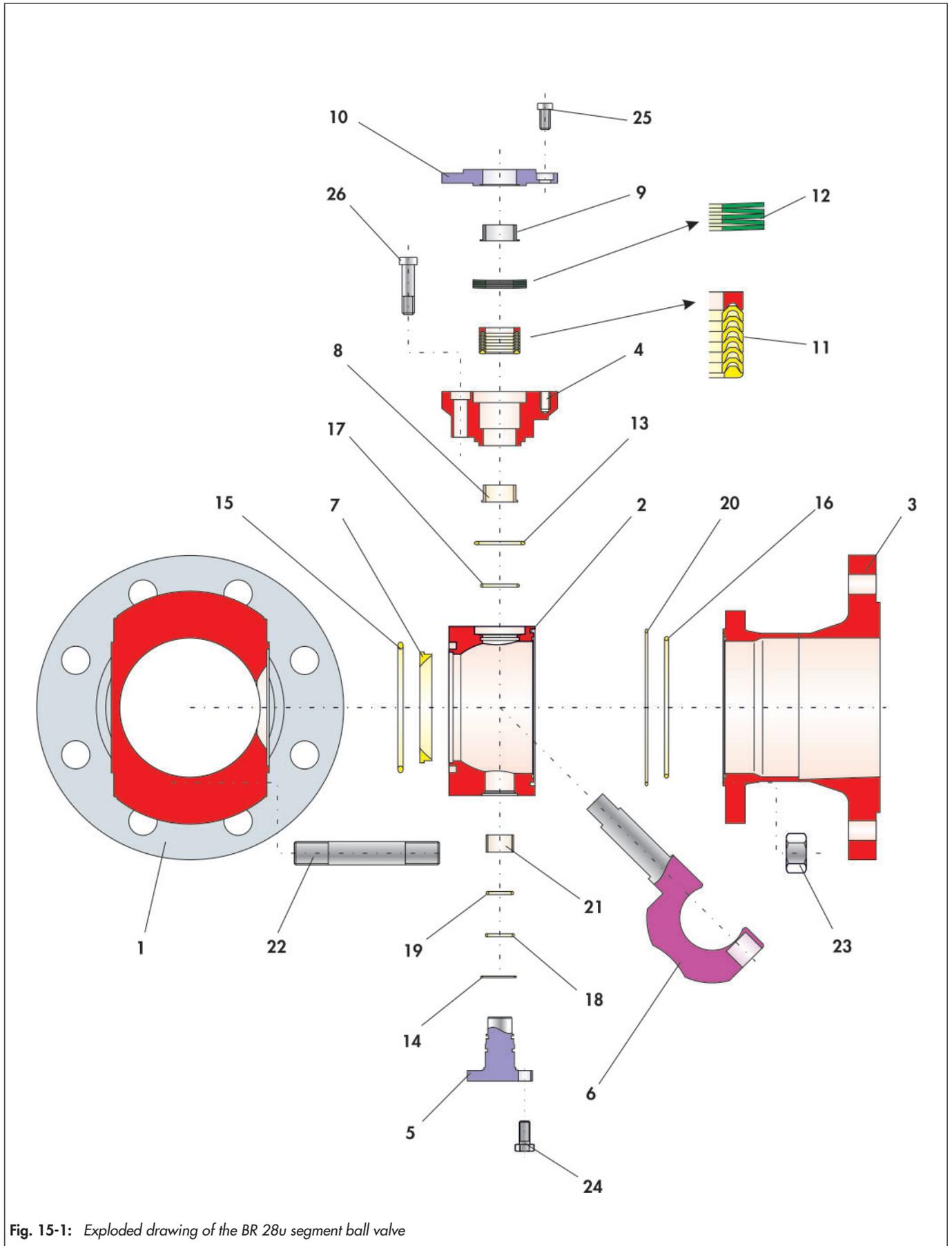
Fig. 15-1: Exploded drawing of the BR 28u segment ball valve
