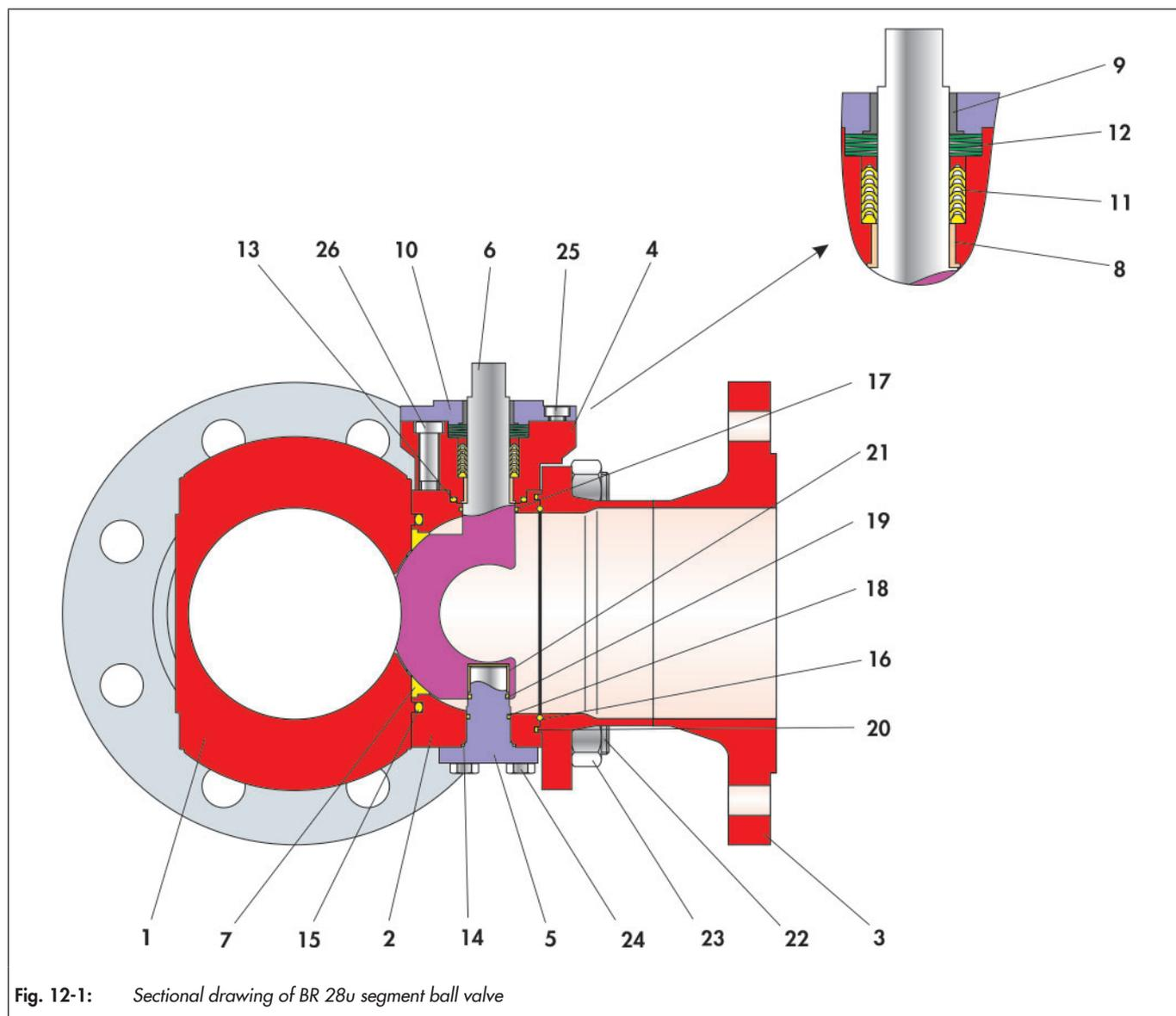
Fig. 12-1: Sectional drawing of BR 28u segment ball valve
