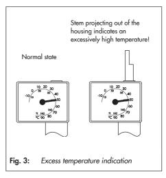
The temperature will exceed the adjusted limit if the valve cannot close due to dirt particles lodged between the seat and plug or due to a defective bellows. In this case, the excess temperature safeguard responds (see Fig. 3). The stem projecting out of the housing indicates a malfunction.
