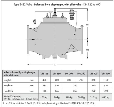
Fig. 6: Dimensions and weights · Type 2422 Valve balanced by a diaphragm
