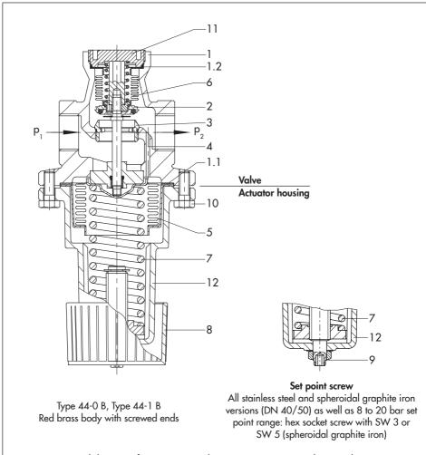
Fig. 9-1: Functional diagram of Type 44-0 B and Type 44-1 B Pressure Reducing Valves
