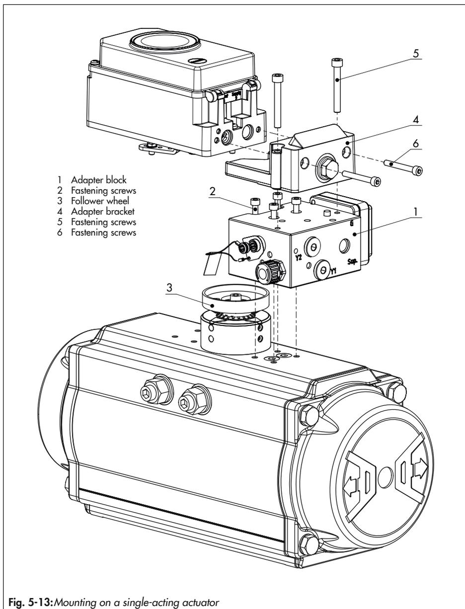
Fig. 5-13: Mounting on a single-acting actuator
