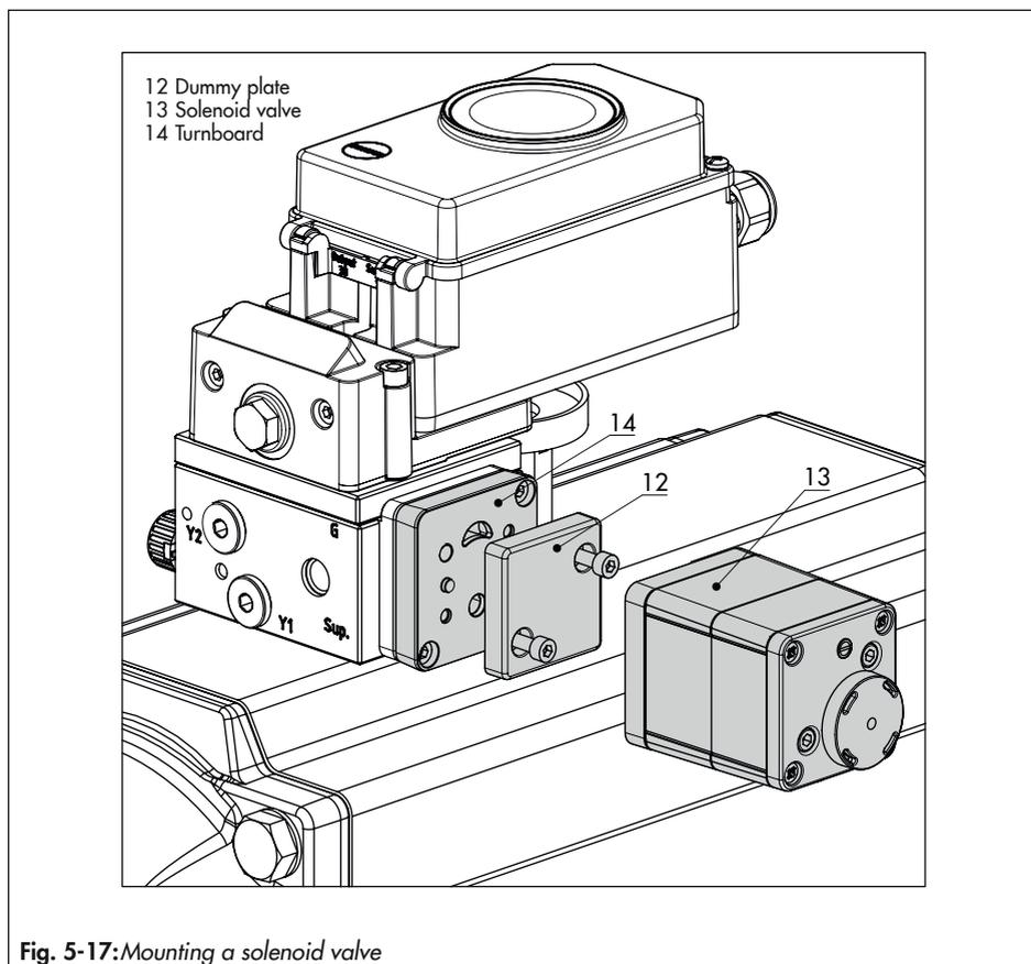
Fig. 5-17: Mounting a solenoid valve
