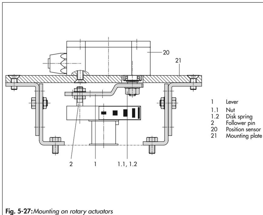
Fig. 5-27: Mounting on rotary actuators
