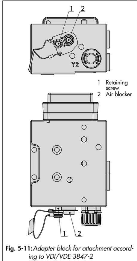
Fig. 5-11: Adapter block for attachment according to VDI/VDE 3847-2
