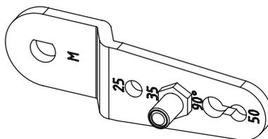
**Fig. 5-3:** M lever with pin position 35
