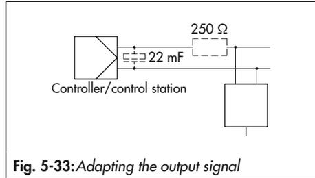
**Fig. 5-33:** Adapting the output signal
