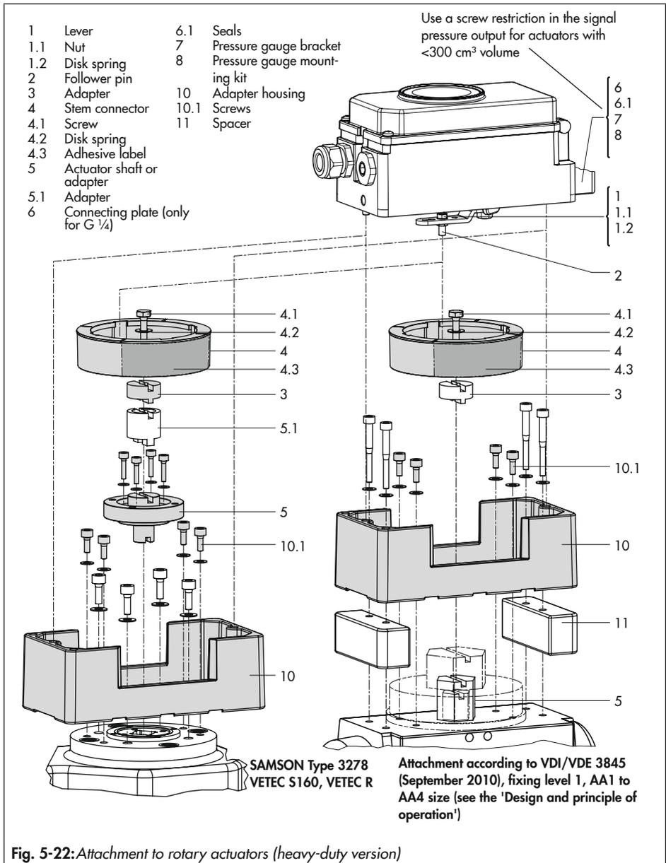
Fig. 5-22: Attachment to rotary actuators (heavy-duty version)
