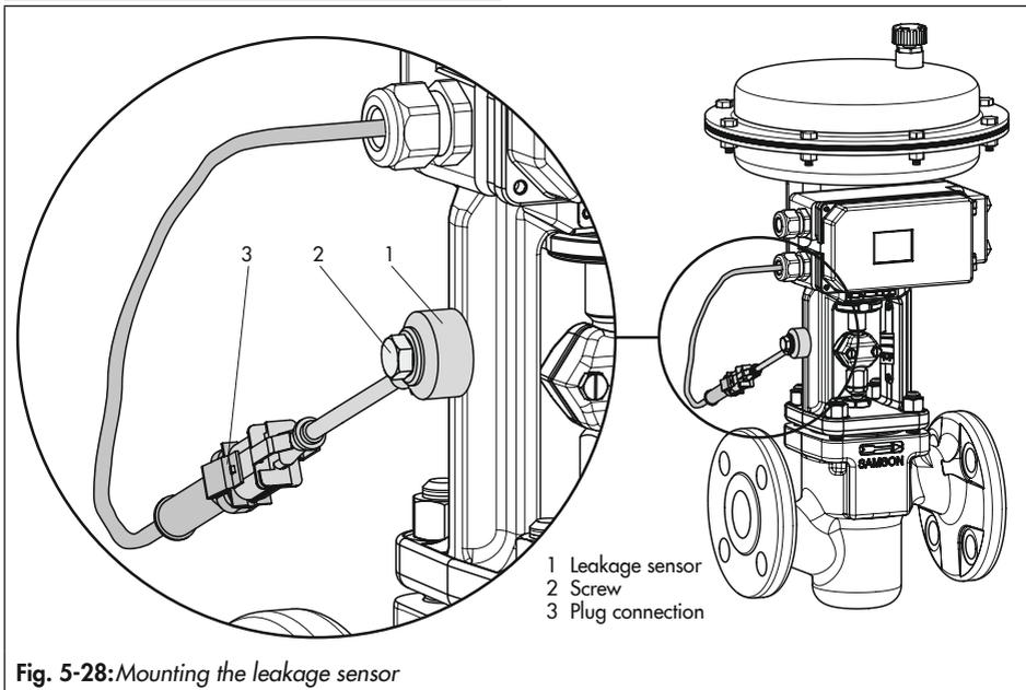
Fig. 5-28: Mounting the leakage sensor
