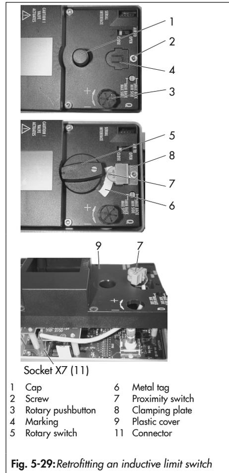
Fig. 5-29: Retrofitting an inductive limit switch
