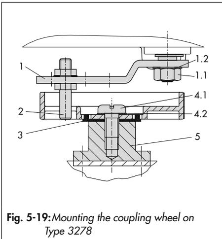
Fig. 5-19: Mounting the coupling wheel on Type 3278
