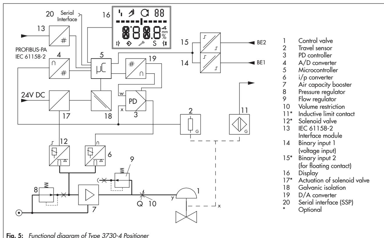
Fig. 5: Functional diagram of Type 3730-4 Positioner
